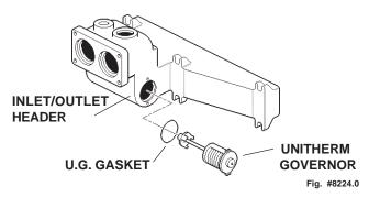
To test the operation of the Unitherm Governor, place in hot water (over 100°F) and watch for movement against spring. If there is not movement, replace unit.
